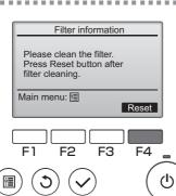
Press the F4 button to reset filter sign.
